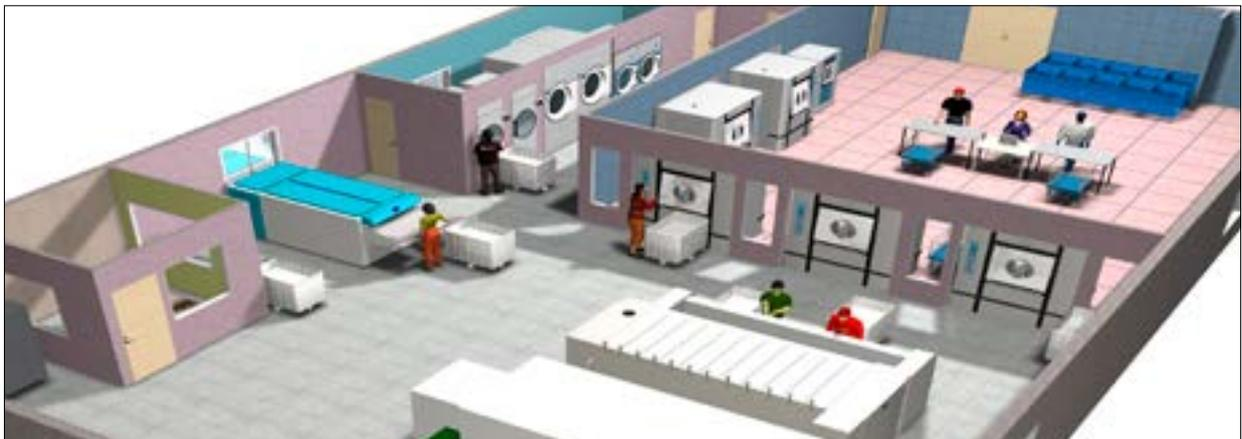
Example of the advanced solution – the innovative Barrier laundry showing equipment in a preferred linen flow.
